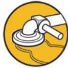
Spread compound and polish at 1,200–2,000 rpm
